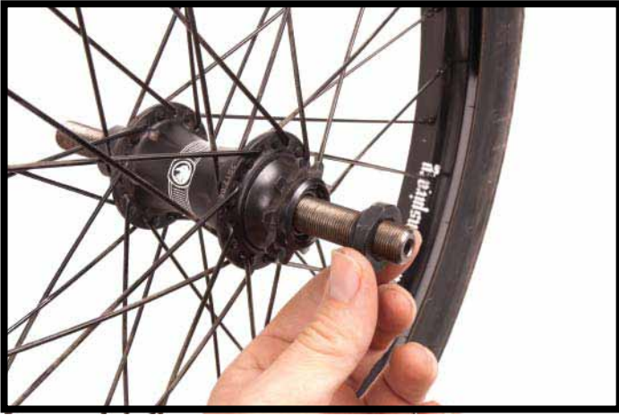
5. Remove the drive-side cone nut.
