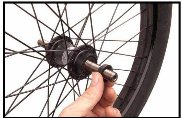
10. Remove the non-drive side cone nut. If snug, repeat the process for the non-drive side lock nut to loosen.
