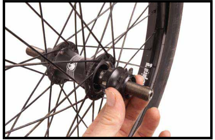
6. Gently pull the driver out of the hub shell. Be careful not to lose any springs or pawls.
