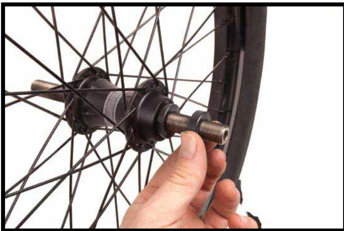
9. Remove the non-drive side lock nut.
