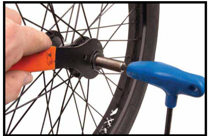
8. Insert the 6mm hex wrench into the non-drive side axle broach and break the non-drive side lock nut free with a 23mm cone wrench.
