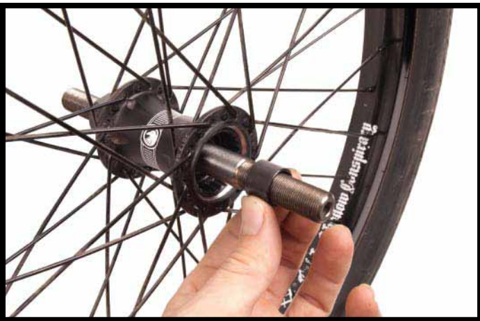
7. Remove the driver spacer from the axle. This spacer may come out when removing the driver.
